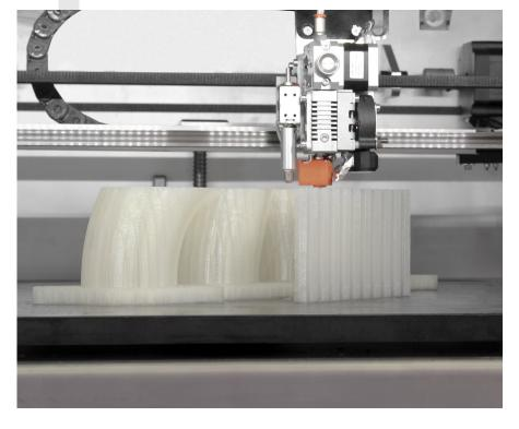
Using the right print bed has a significant impact on print quality. Especially when printing large objects. Having an ultra-flat bed with great product adhesion will reduce a lot of basic printing problems that you may face. To achieve this, we use a Granite print surface for a number of reasons.
